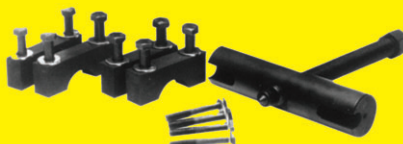
Yoke Puller for H.D. truck application with carrying case. Works on full and half round yokes found on Spicer, Spicer & Meritor and Meritor (Rockwell). Use with 1/2" impact wrench. TGT-10803
