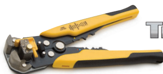
Self Adjusting Wire Stripper/Cutter/Crimper Automatically adjusts to strip 24 - 10 AWG wire and cable. Crimps 22 - 10 AWG insulated and non-insulated wire terminals. Crimps 7 - 8mm ignition terminals. TTN-11475
