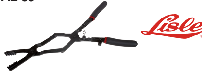
Long Reach Hose Clamp Pliers Overall length of 17" provides extra long reach. Cross-cut tip design grips most hose clamps from multiple angles. Ratcheting lock mechanism holds the clamp in an open position for hands-free use. Dual material grips for comfort. LIS-17000
