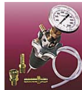
Connect Mityvac's universal cooling system adapter to most standard cooling system testers - transforming your dedicated pump into a versatile tool. Multiple fittings allow for interchange between Mityvac's universal adapter and user's standard adapter. MV-4521
