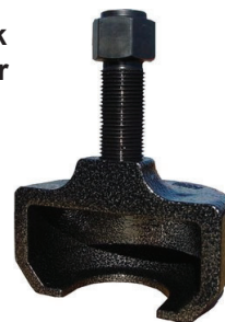
Heavy Duty Truck Pitman Arm Puller Can be used with 3/4" impact guns. For "Sheppard M100" style pitman arms. TGT-10385
