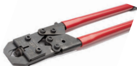
Heavy Duty Adjustable Cable Crimper with 50 different crimp settings, works on 6 gauge to appx 5/8" cable. Exerts equal pressure on all contact points. EZ-B795
