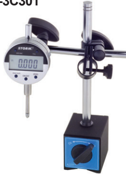
Digital Indicator Set 0-1 Inch (0-25mm) • On/off magnetic base • Digital display • Reads in inch, metric and fractional inch STO-3D105
